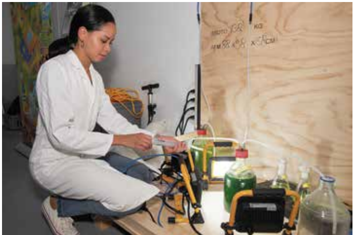
Bonairean Rocca Chinon, PHD Biotechnology student at Wageningen University takes a sample of the algae growing for the photo bioreactor at the laboratory in Bonaire.
