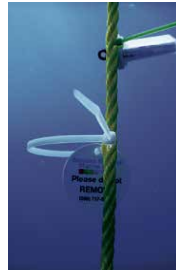
HOBO sensor (depth 5m) + STINAPA tag to inform divers not to remove the sensors. The sensors are installed pointing upward to catch as much light as possible. They are also cleaned of algae and other things that might be growing on them every week.
