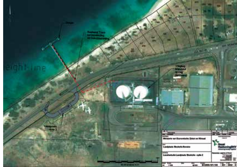
Emergency Plan A: The BIA fuel pier at the airport. The red line shows the existing arrangement for transporting jet fuel from the receiving pier to storage tanks. A similar facility will be built for bringing ashore heavy oil, which then would be trucked directly to Contour Global.
