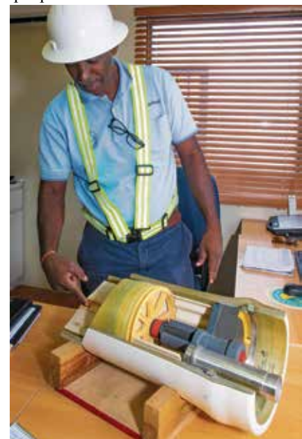
Edson Martinus shows cross section of reverse osmosis pipe.
