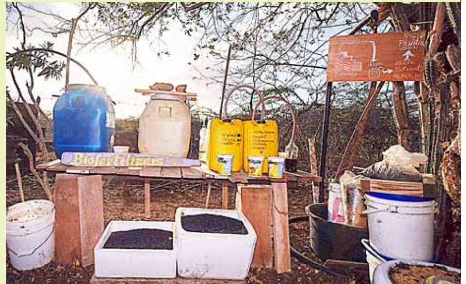
The setup to make cooking gas
