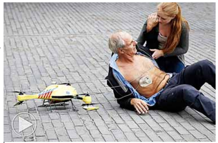
A drone carrying heart defibrillator (AED) can be dispatched fast to save lives
