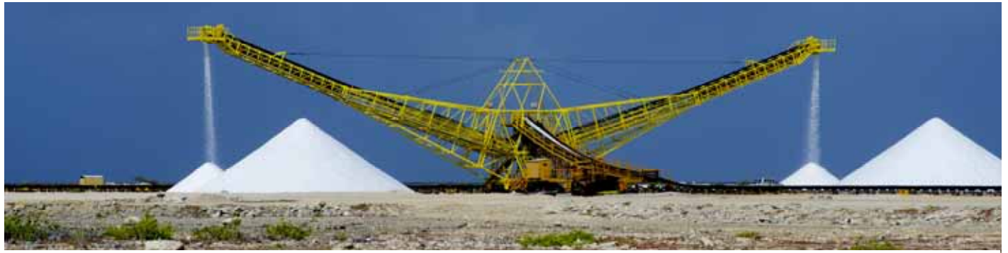
Looking like some creature from another universe, the mobile conveyor builds the crystal cones of salt
