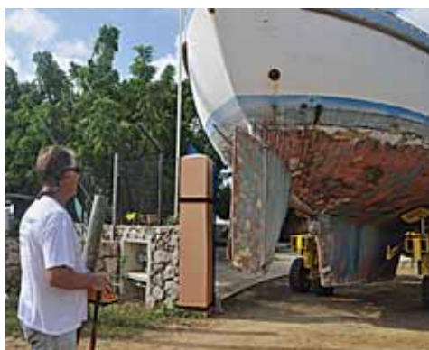
Maneuvering via radio control
