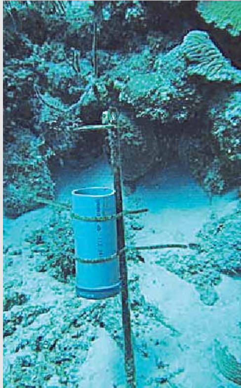
One of the CIEE sediment traps. If you see one of these while diving, please don't disturb it.
