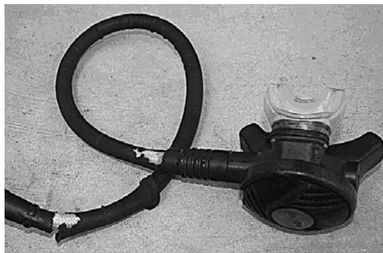
This picture shows a hose outer rubber cover – or lack thereof. Although not recommended, this hose is still being used daily and has functioned this way for years!
