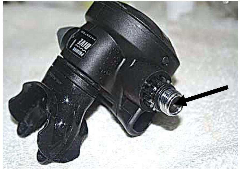
A typical 2 nd stage. Orifice is located inside the chrome “tube” on the right side of this 2 nd stage.
