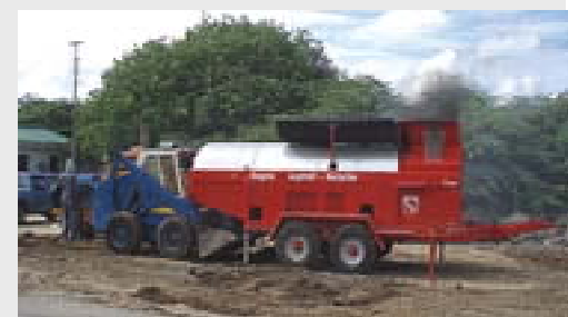
Asphalt recycling machine on Kaya Gob. Debrot
