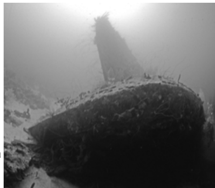
The rudder used to be sideways. It has tilted upwards with the roll of the ship as it collapsed.
