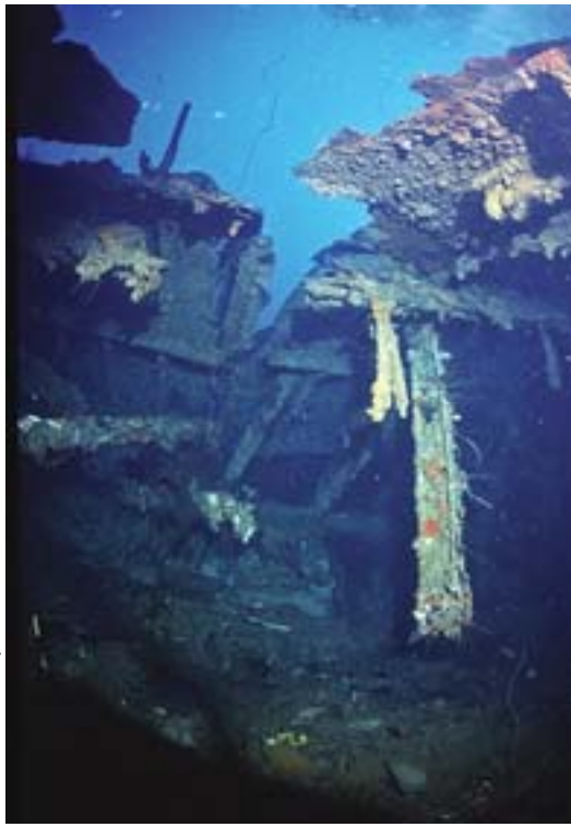
Inside the Windjammer you can see the gaping new crack and the sheared metal framing.
